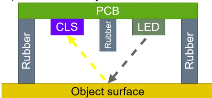
Figure 3. Detecting non-self-illuminating objects
