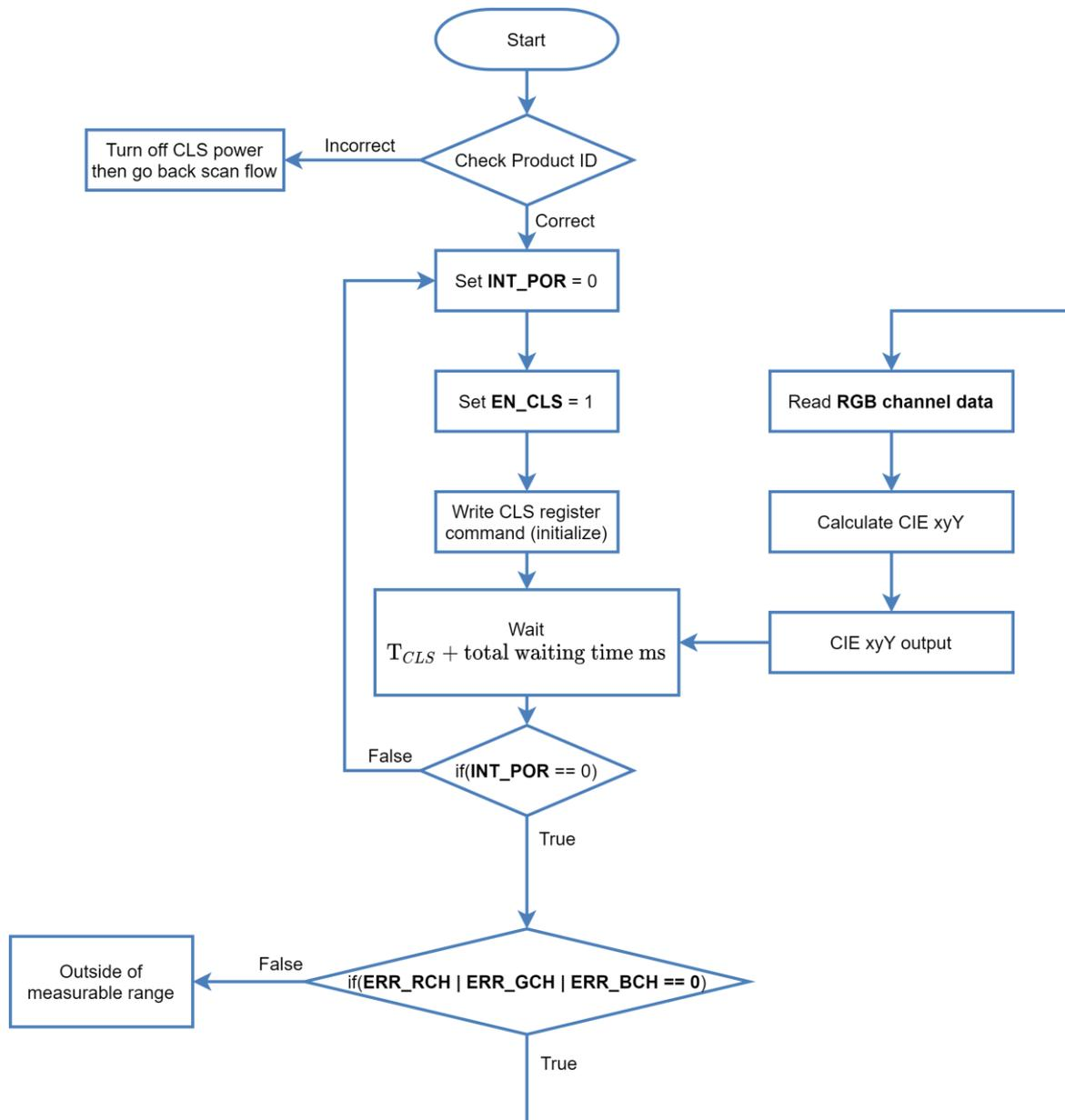
Figure 8. Firmware design flow chart
