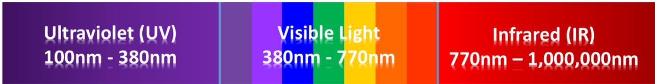
Figure 5. Electromagnetic wave classification
