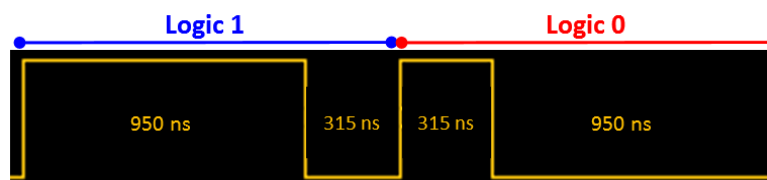
Figure 5. Logic 0 and Logic 1 waveform
